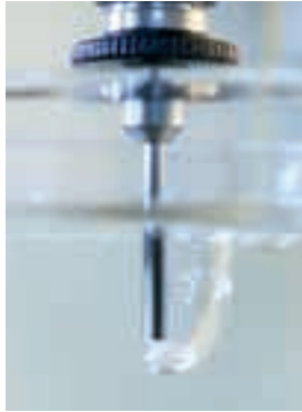
Figure 4: Measurement of dynamic surface tension with the bubble pressure tensiometer
