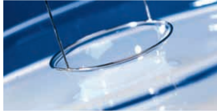
Figure 5: Measurement of static surface tension by the du Noüy method
