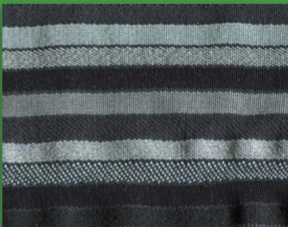
**Low or on-tone staining of multifiber strip during dyeing**
