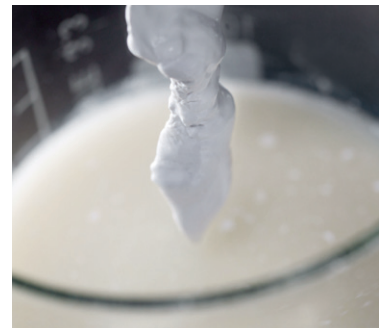
Paint with strong sedimentation
