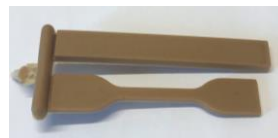
80% PLA, 20% fibers, injection moulded sample
