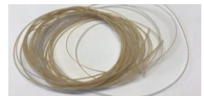
80% PHB, 20% fibers, monofilament
