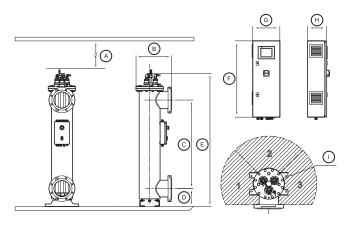
1 Minimum distance to ceiling or wall, depending on installation, for service.
