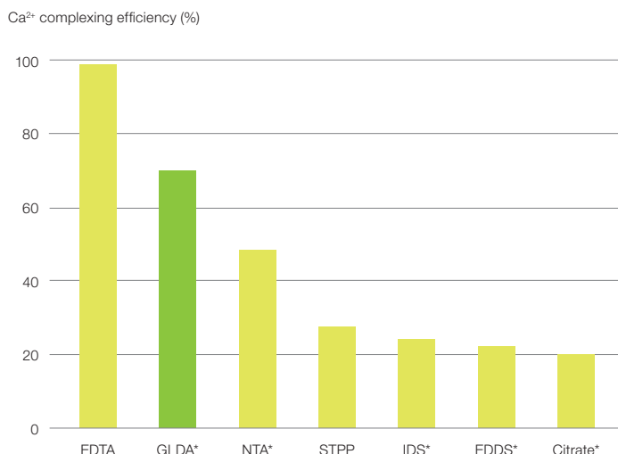
Figure 10 The \text{Ca}^{2+} complexing efficiency of various chelating agents in competition with Hydroxy Naphthol Blue at pH 11-12. * Readily biodegradable chelating agents.
